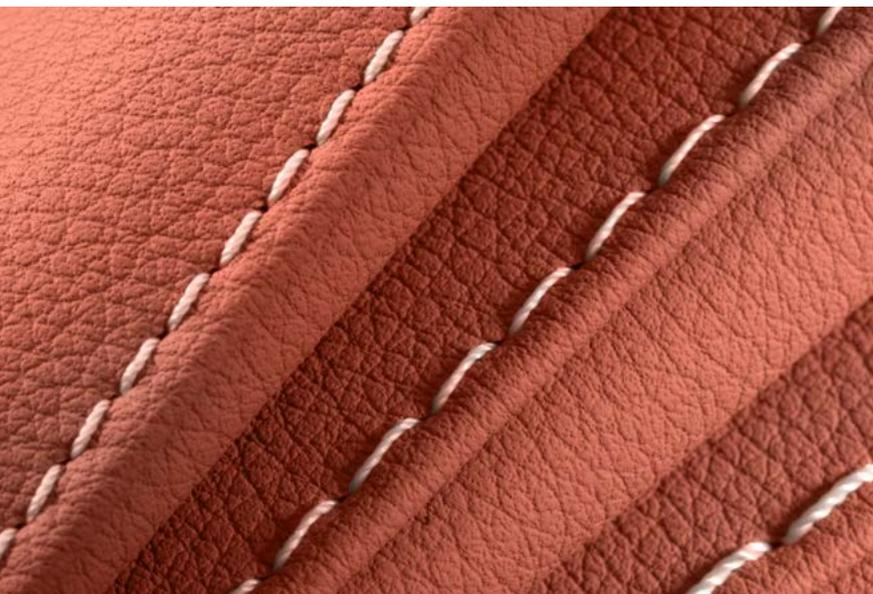
Using sewing needle diameters that are too large on thin leather materials creates unnecessarily large puncture holes. These can weaken the leather seam or even cause the seam to tear. However, if a needle size that is too small is used for the sewing thread, the thread material may bunch up or even break.
