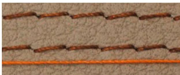
Standard corespun thread: the red wine test causes permanent discolouration – here you can see the original sewing thread in comparison.
